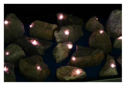
The project uses Laser-Induced Breakdown Spectroscopy (LIBS) to sort out components in refractory materials. The bright spots in the picture show the energy generated by the laser to facilitate element mapping.
