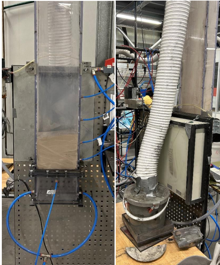
Figure 14 Experimental setup. Fluidization column with air inlet and pressure sensors. To the right, outlet trough filter bucket.
