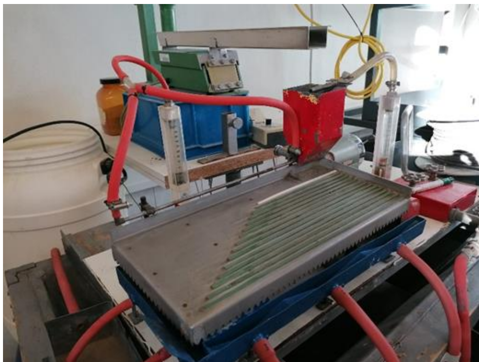
Figure 43 Lab shaking table at the Chair of Mineral Processing, Montanuniversitaet Leoben.
