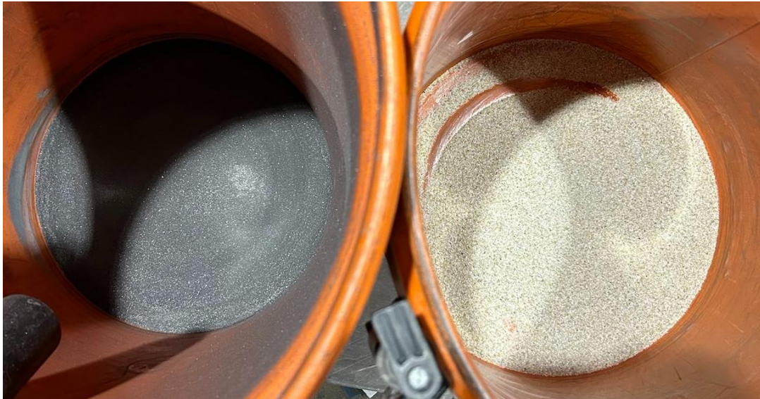
Figure 28 Fine (left) and coarse (right) fraction after separation in Test 15.
