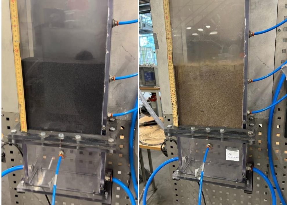
Figure 22 SCL (left) and CRK (right) both 0.25-0.5 mm at 0.095 m/s.
