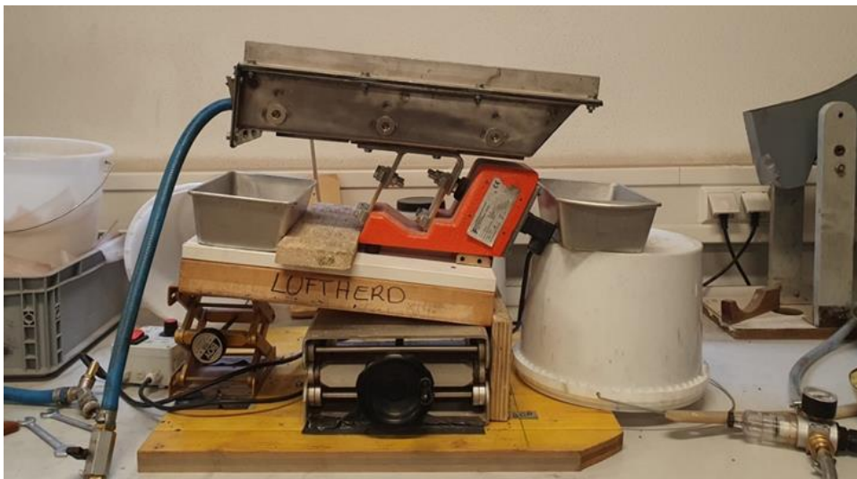
Figure 42 Air separation table at the Chair of Mineral Processing, Montanuniversitaet Leoben.
