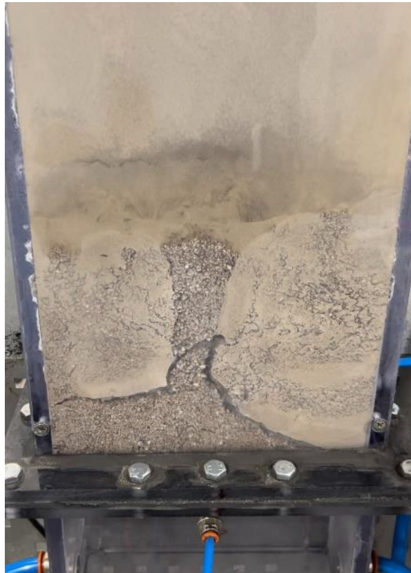
Figure 21 CRK leftover material 0-5 mm while fluidization experiment at air velocity 0.24 m/s
