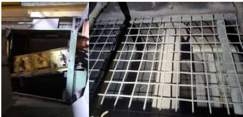
Figure 11: Circular vibratory screen with two screen decks
