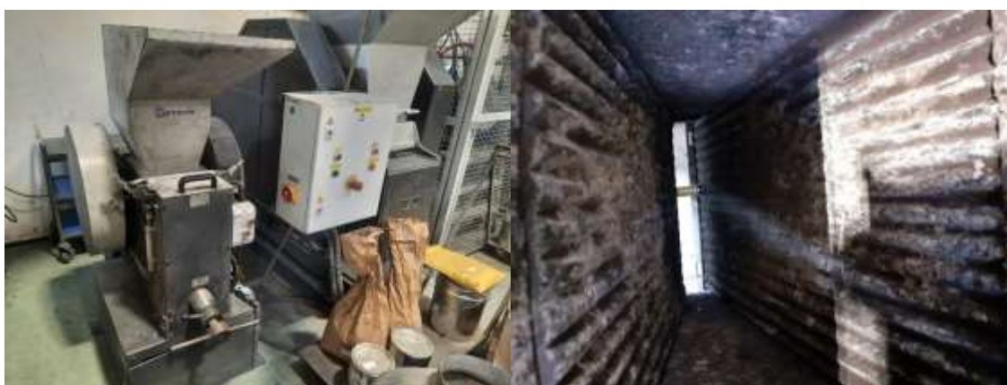
Figure 15: Laboratory crushing tests – jaw crusher
