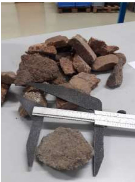
Figure 22: Analysis of particle size and particle shape distribution – particle shape slide gauge
