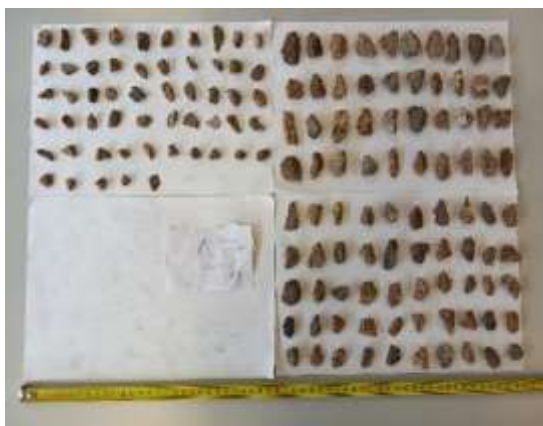
Figure 23: Analysis of particle size and particle shape distribution – Sample A cone crusher, subsample fraction 20/10 mm
