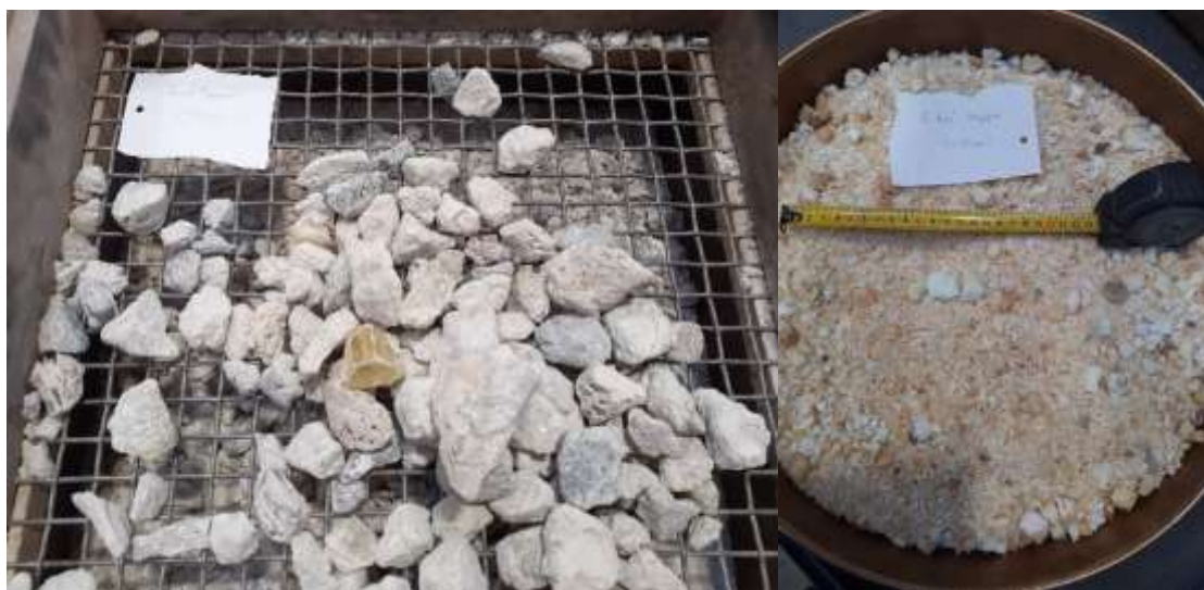
Figure 13: Laboratory crushing tests – particle size classes (left: fused magnesia >20 mm, right: sintered magnesia 0–40 mm)
