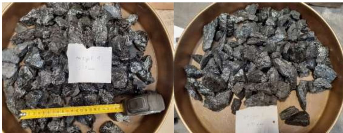
Figure 14: Laboratory crushing tests – particle size classes (left: Hercynite 1 >20 mm, right: Hercynite 2 >20 mm)
