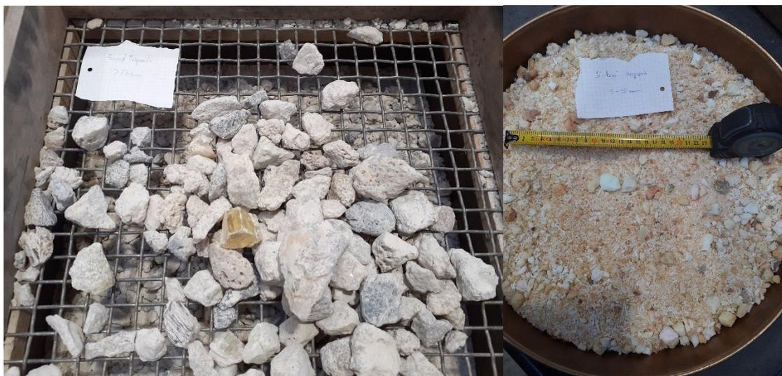
Figure 13: Laboratory crushing tests – particle size classes
