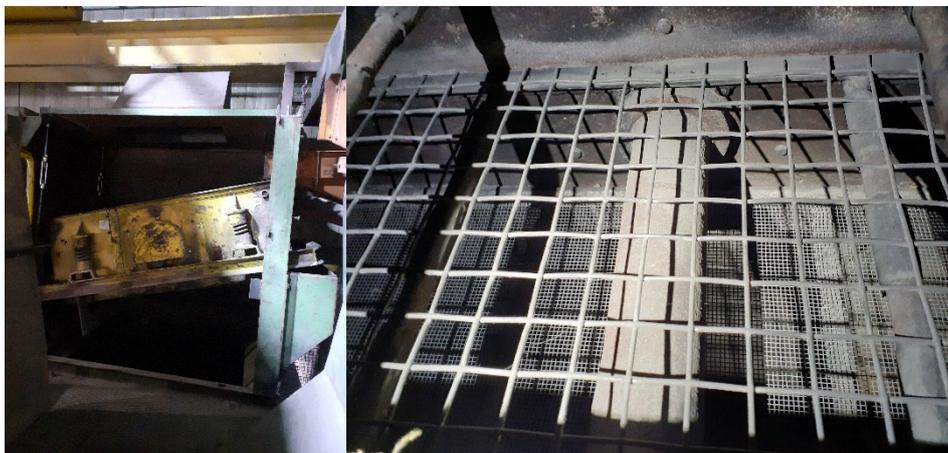
Figure 11: Circular vibratory screen with two screen decks
