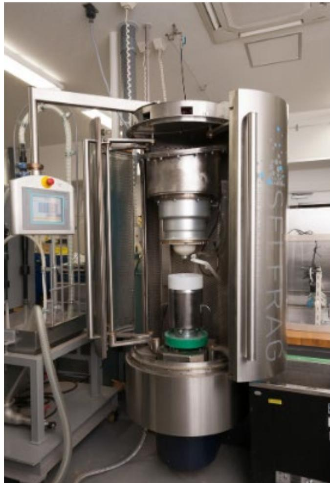
Figure 5: EDF lab equipment at MUL [5]
