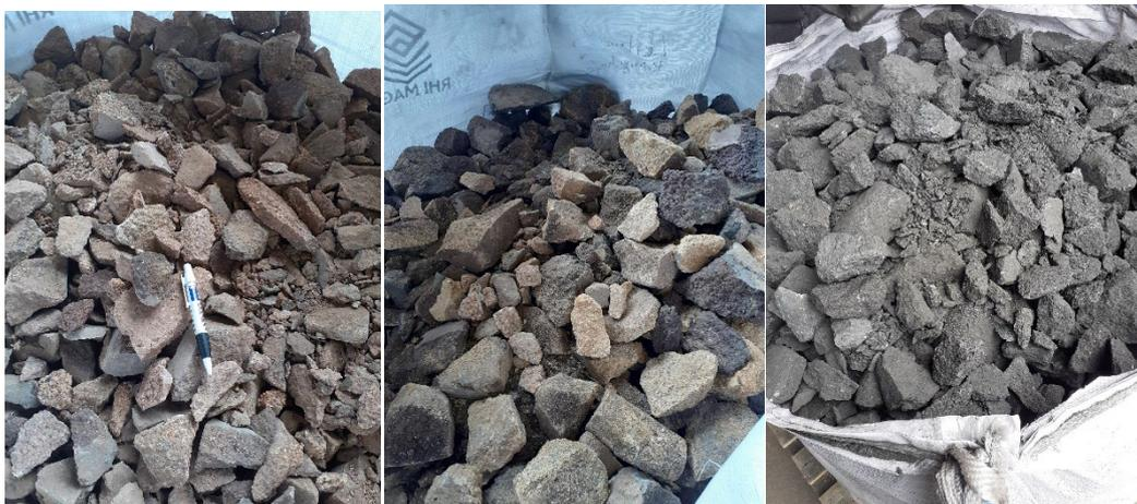
Figure 8: sample A (Hercynite), sample B (Hercynite) and sample C (MgO-C), from left to right.
