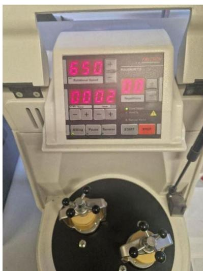
Figure 21: Pulverisette vacuum ball mill
