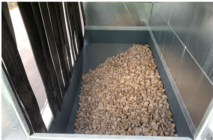
Figure 8: Feed hopper with maximum achievable fill level; left in the image: vertical opening for filling
