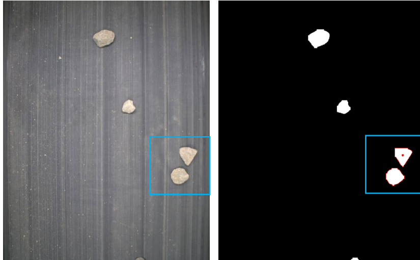
Figure 7: Left: Original image; Right: Representation of particles considered critical (red border: Inter-particle Distance Too Small; Red Dot at Centroid: Distance to Edge Too Small)
